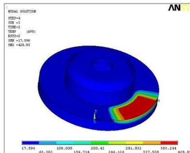
At t = 2.0 sec,  $T_{max} = 428.95 \text{ } ^\circ\text{C}$
